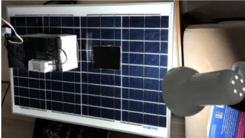
Figure 4.22. Photodetector test device without UV LED.
