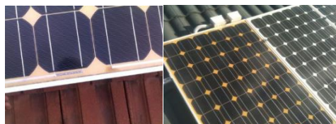
Figure 2.19. Browning and Yellowing Fault [80].
