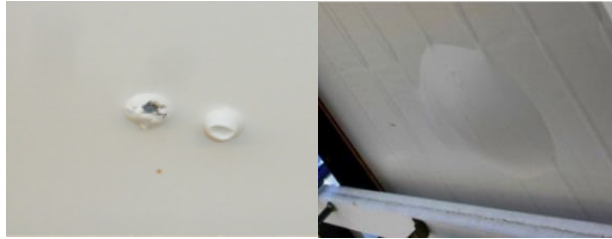
Figure 2.20. Back Sheet Blistering [80].
