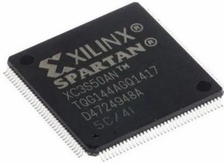
Resim 3. 2 XILINX XC3S50AN-4TQG144C model FPGA ipi (İnt. Kyn. 5)
