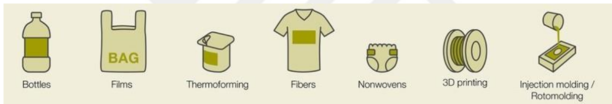
Figure 4 Main PLA Application Areas [69]
