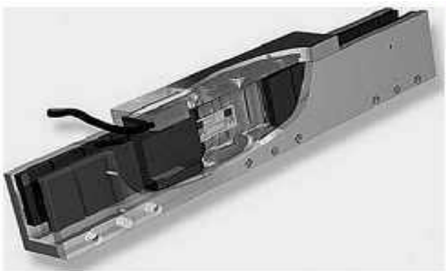
Figure 1.11 : Flat double-sided PM LBM with moving coil [17].
