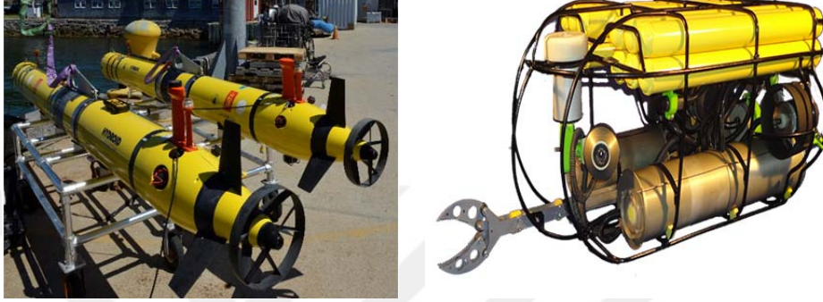
Figure 1.3. Examples of AUV (Anonymous, 2019e) and ROV (Anonymous, 2019b)
