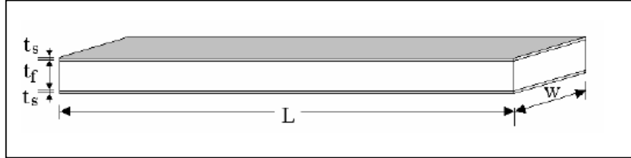
Figure 4.4 Geometry of flat sandwich beam
