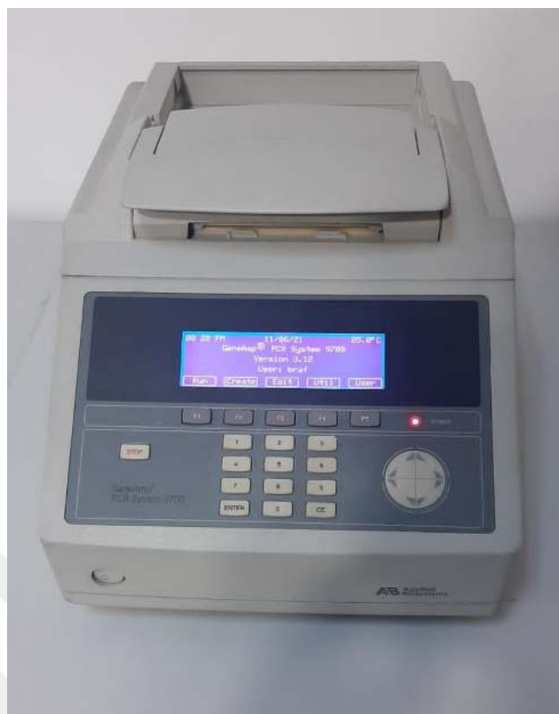
Figure 2.4. GeneAmp PCR system 9700/USA used for the analysis of the samples
