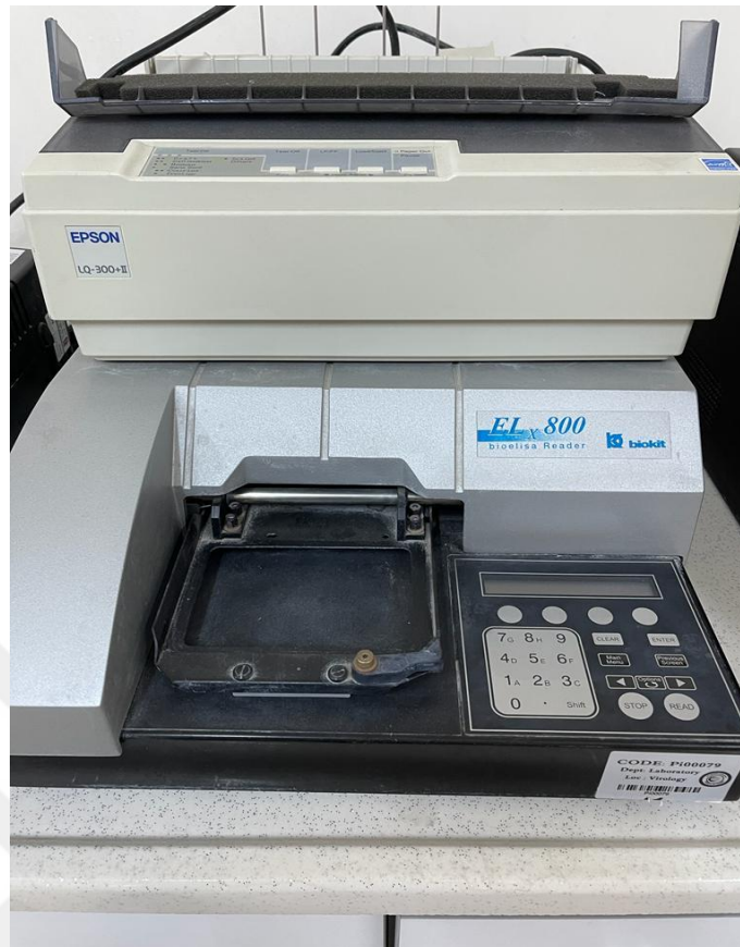
Figure 2.3. Biotech ELx 800-Epson/USA used for the detection of RV antigen in stool samples
