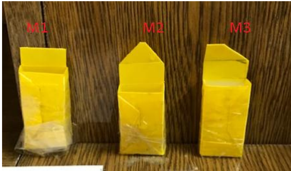
Figure 3. 12 M1, M2 and M3 samples which are kept in a cool environment for curing after mixing separately to certain sizes.
