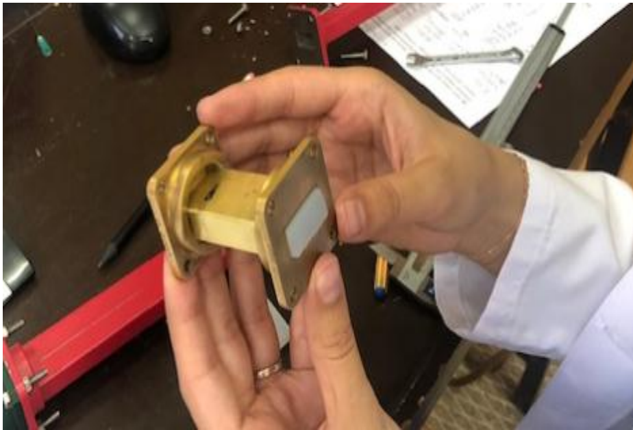
Figure 3. 17 We put the sample we prepared in the rectangular waveguide
