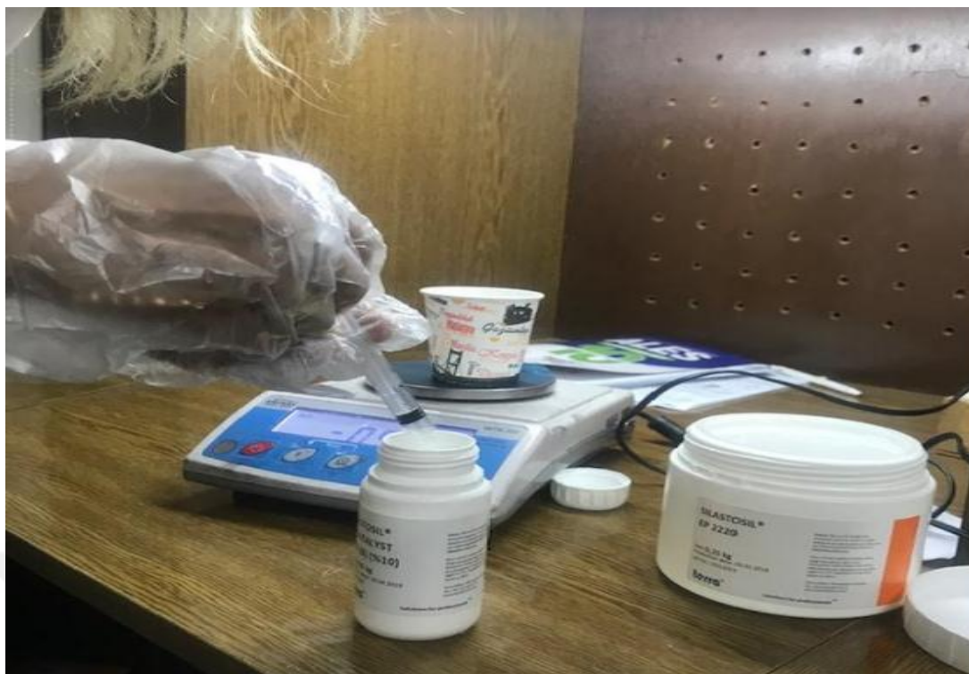
Figure 3. 6 10% catalyst base mixture for M1
