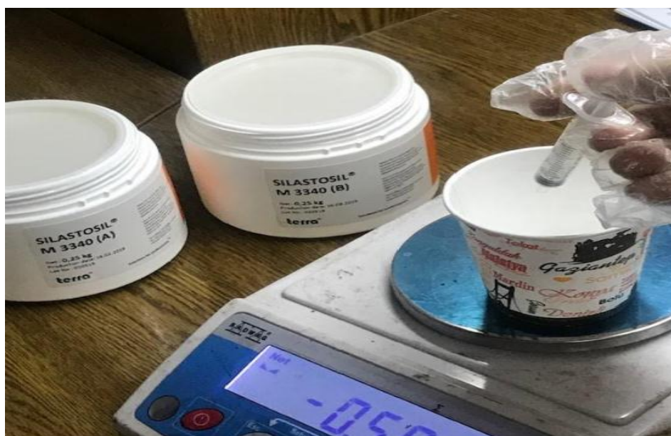
Figure 3. 11 50% catalyst base mixture for M3
