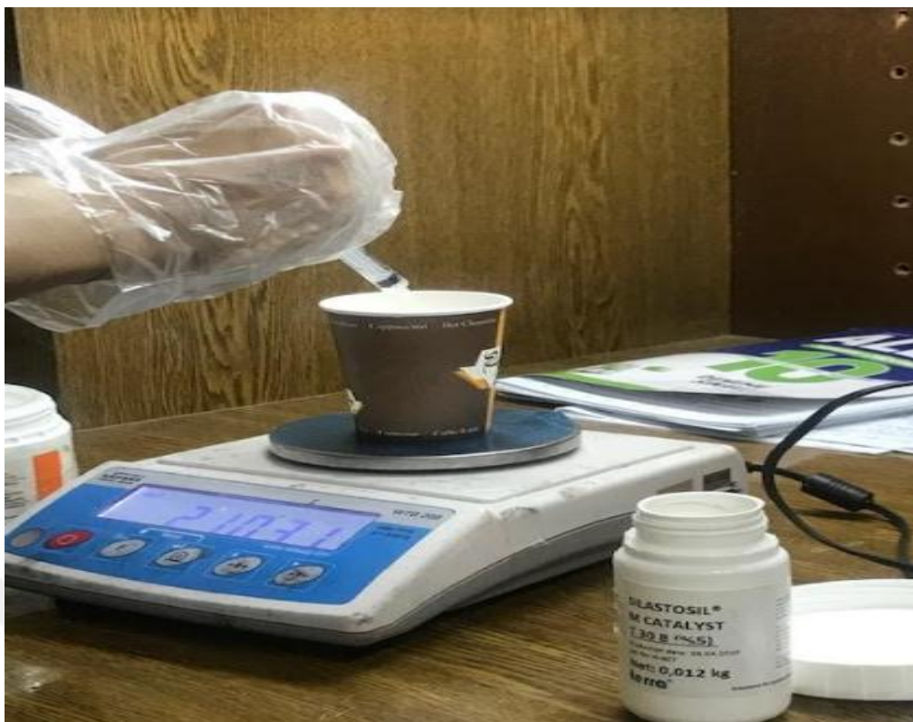
Figure 3. 8 5% catalyst base mixture for M2
