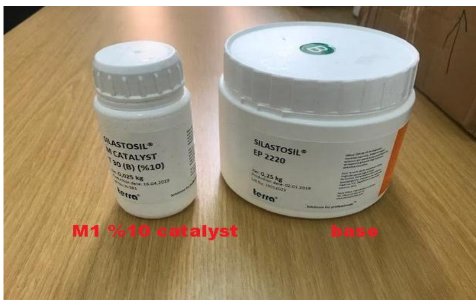
Figure 3. 1 Base and catalyst of sample M1
