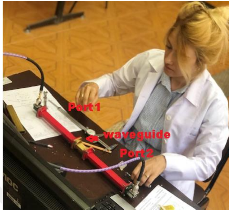
Figure 3. 16 Circuit for calibration of empty rectangular waveguides located between two ports
