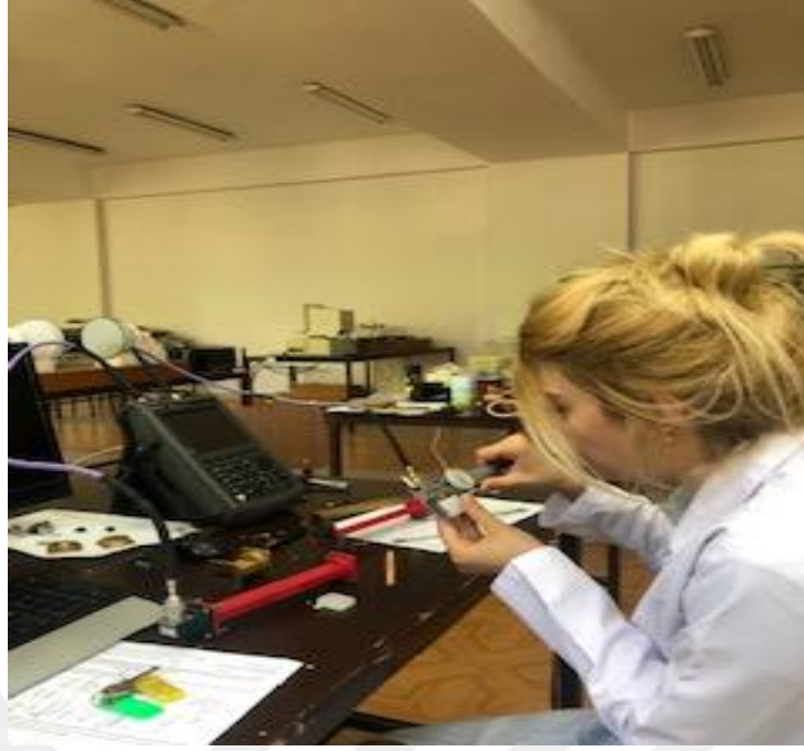
Figure 4. 2 We measured the size of the sample with a caliper and found 25.5 cm, then we made the necessary calculations by replacing L with this value.
