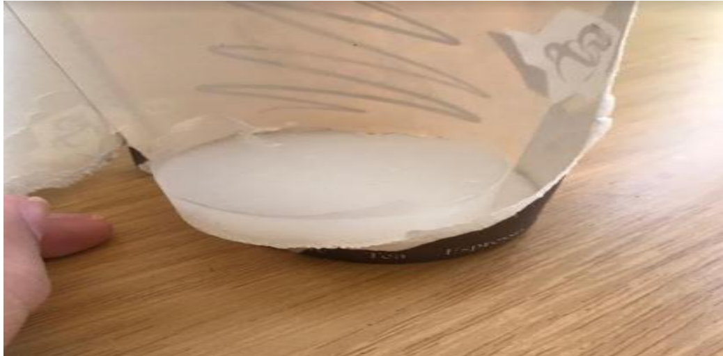
Figure 3. 7 A sample of silicone that cured in cardboard
