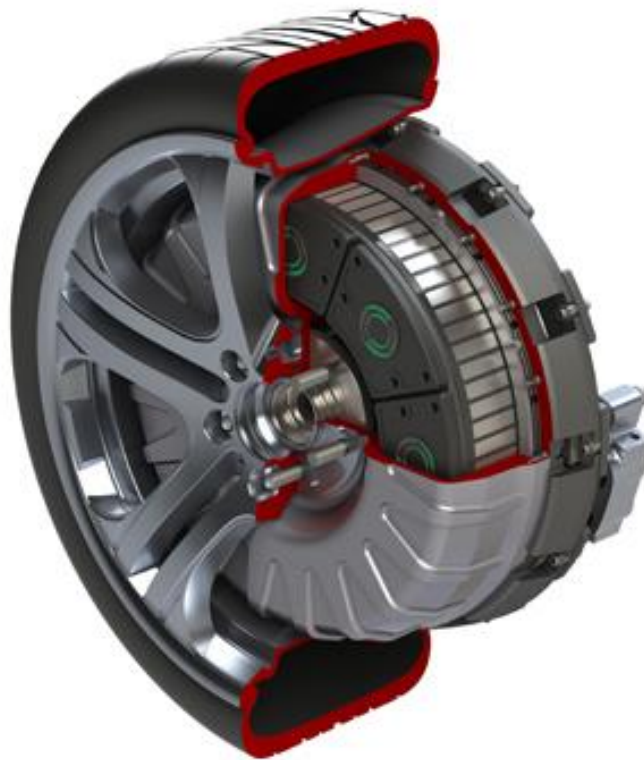
Figure 2.4 Protean Electric HUB Motor Cut-away (Protean, n.d.)
