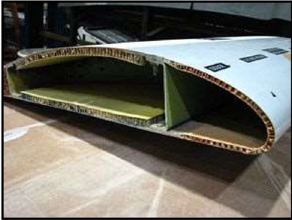
Figure 1.10 Application of Sandwich Composite Material on Aircraft Wing [32]
