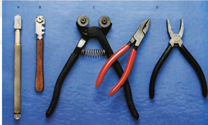
Görsel 3.10. A-Hazneli Elmas, B-Elmas, C- Kesme Pensesi, D- Penseler (Beveridge, Domenech, Pascual, 2005, s.44).
