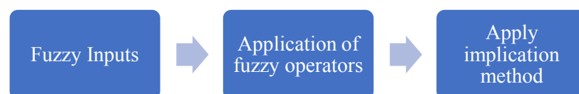
Figure 3.6. Rule processing algorithm
