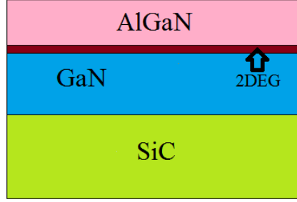
Figure 3.9: General HEMT device structure from side view
