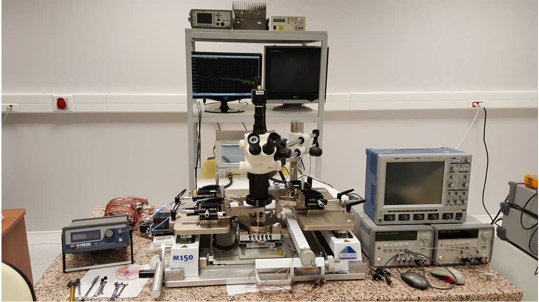
Figure 3.6: Small Signal measurement setup
