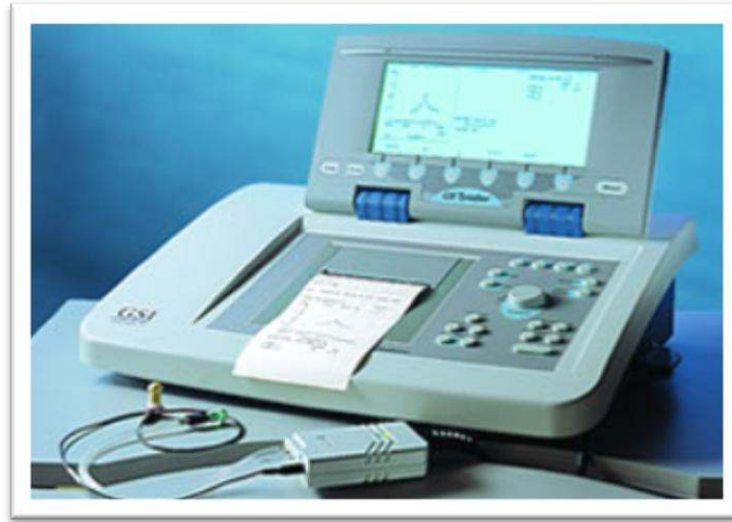
Şekil 6. GSI (Grason-Stadler Inc.) Tymptar Middle Ear Analyzer Version 2 (86).
