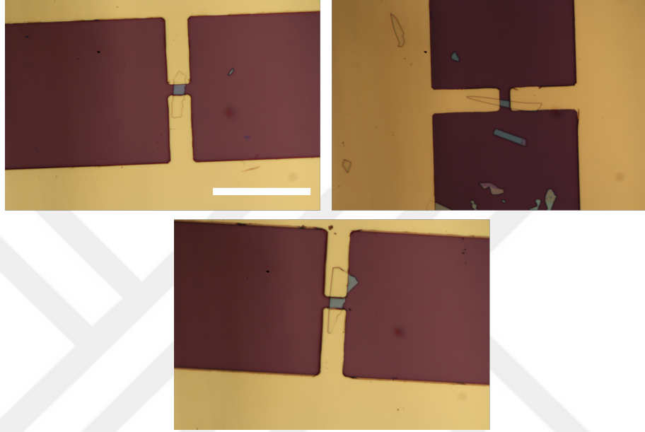
Figure 3.5: Optical micrographs of the fabricated devices top contact devices using optical lithography. Scale bar is 30\mu\text{m}
