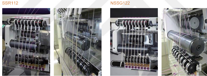
Comparison of yarn course of each type of DSCS
