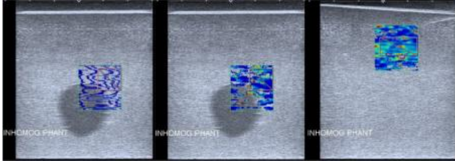
Figure 4.6. Propagation speed direction (left), color map by separating the areas having different elasticity properties (middle), and color map of the background only (right)
