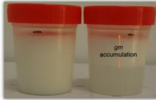
Figure 3.2. Left: uniform, Right: failed gel phantoms including gm
