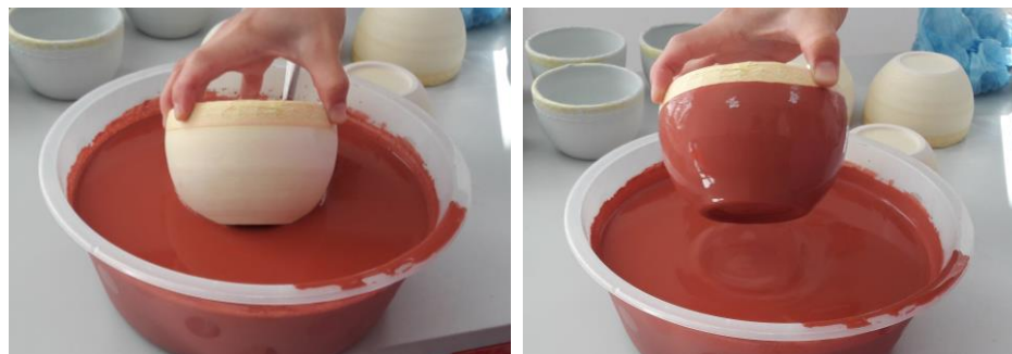
Figure 65: Glazing process (Asmahazi Osmera, 2018)
