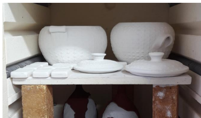
Figure 67: Products ready for glaze firing (Asmahazi Osmera, 2018)
