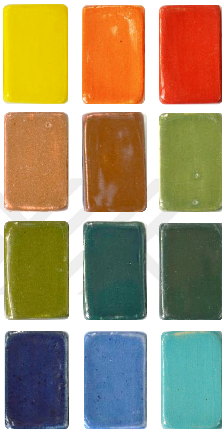
Figure 70: Engobe colours applied onto final products (Asmahazi Osmera, 2018)
