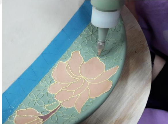
Figure 61: Slip trailing decoration process (Asmahazi Osmera, 2018)
