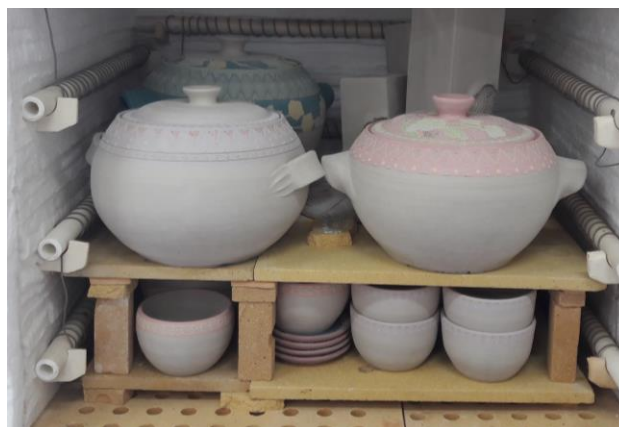
Figure 63: Products ready for bisque firing (Asmahazi Osmera, 2018)
