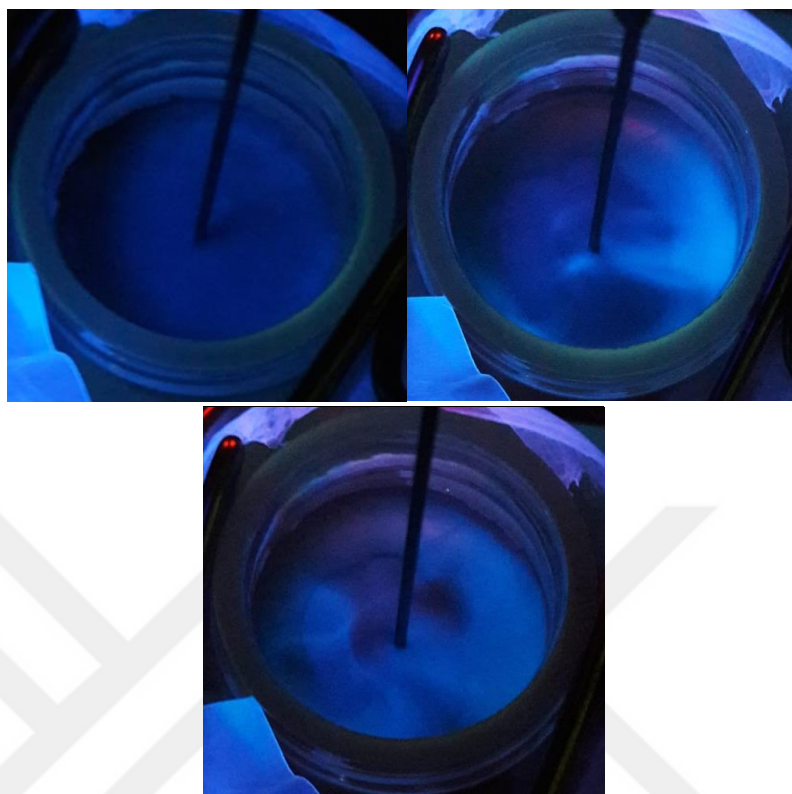
Figure 3. 3 Bare metal with 0.1 M Na 2 SO 4 containing 100 mg/L quinine, the initial picture without any fluorescence and the emergence of fluorescence with applied potential.
