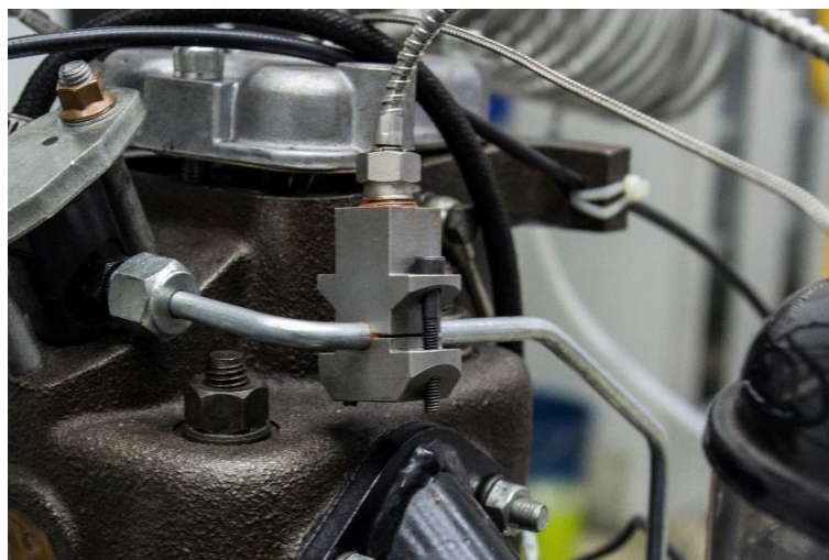
Figure 2.11. Fuel line pressure sensor
