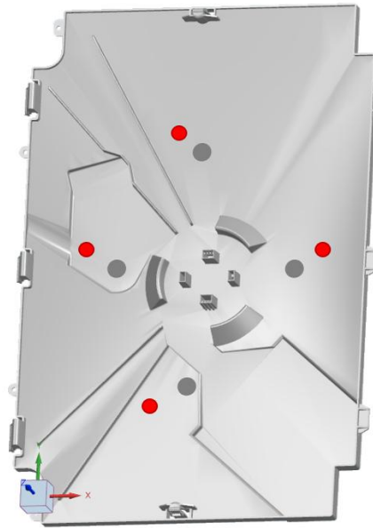
Figure 5.3: Placement of cavity pressure sensors on the dishwasher bottom cover part with sensor locations marked in red and valve-gate positions highlighted in gray.
