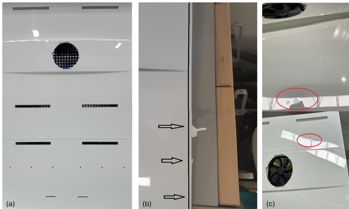
Figure 6.3: Visual inspections of the refrigerator's inner beyond cover, (a) example of quality standards, (b) example of flashes, (c) example of gate blush
