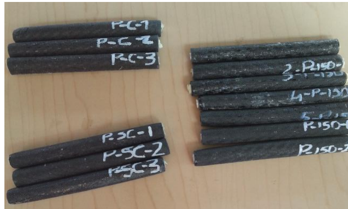
Figure 5.7 : Torsion test specimens: base, middle and separate with 0.5 wt% CNT-ECNs mats.
