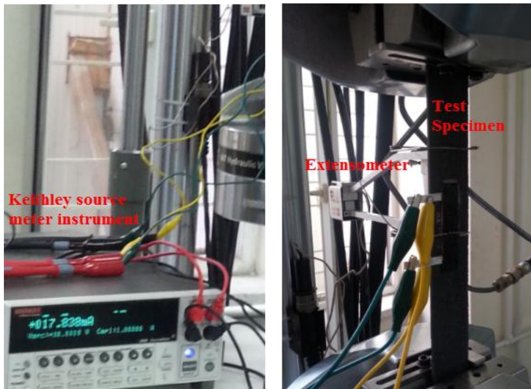
Figure 4.11 : Test system for in situ diagnostics at tensile testing.
