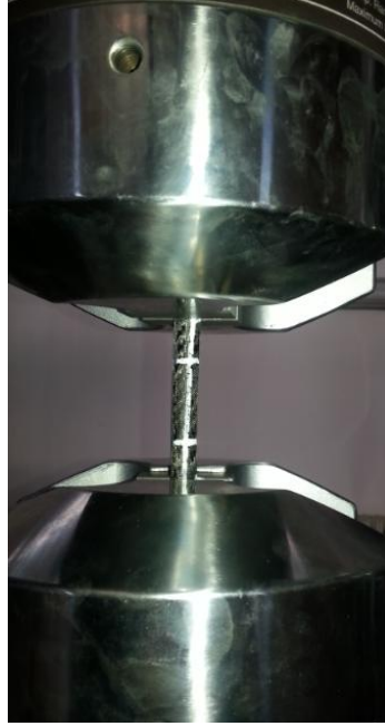
Figure 5.5 : Torsional test of cylindrical hollow structure composite.
