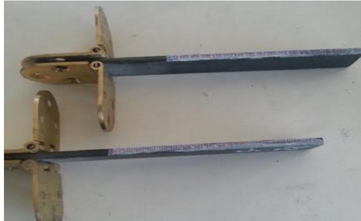
Figure 5.13 : Mode-I Mode II mixture tests specimens.
