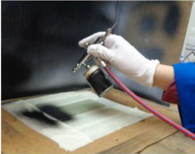
Figure 2.25 : Spray deposition of CNT film onto glass fibers [70].
