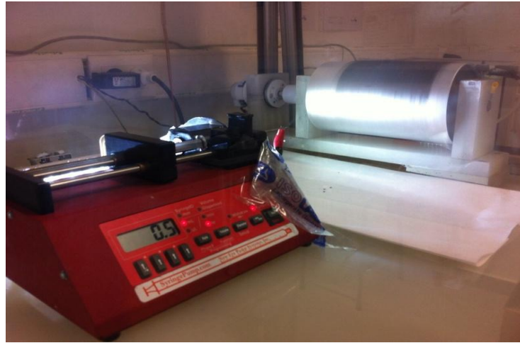
Figure 5.1 : Electrospinning set-up for carbon fiber prepreg composite.
