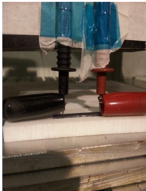
Figure 4.3 : Electrical conductivity measurement setup of CNT-PNCs.
