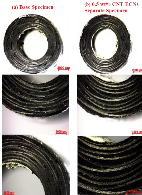
Figure 5.11 : Optic microscope images of cross section of (a) base specimen, (b) 0.5 wt% CNTs reinforced separate specimen after torsion tests.
