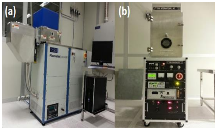
Figure 3.1 : (a) Oxford Instrument Plasma Lab System 100 plasma enhanced CVD (PE-CVD), (b) Torr International Inc. electron beam evaporation technique (E-beam)
