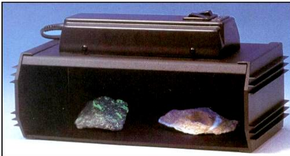
Figure 2.3 Gemmological ultraviolet lamps for measuring the long and short photoluminescence reactions of Biga chrysoprase.
