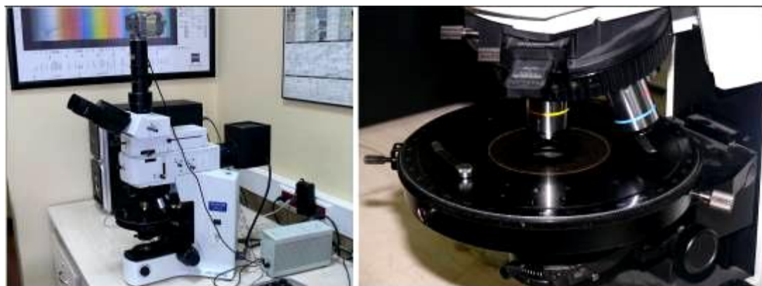
Figure 2.4 Olympus BX41 binocular polarizing microscope with a high intensity 6V, 30W halogen light source combined with U-CPA and U-OPA optical systems, used in this investigation.
