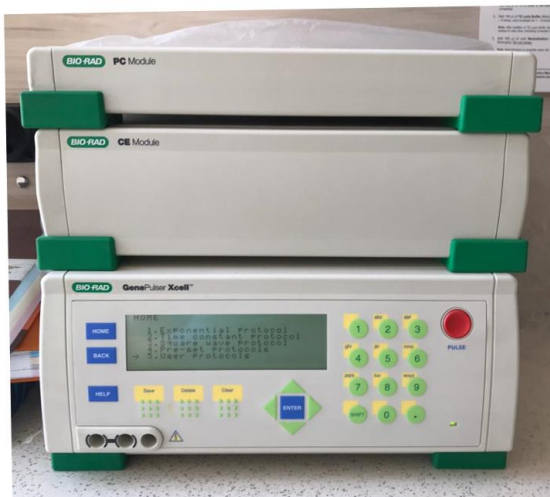
Figure 3.5. Electroporation device used in transformation with Agrobacterium competent cell
