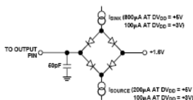
Figure 1. Load Circuit for Access Time and Bus Relinquish Time
