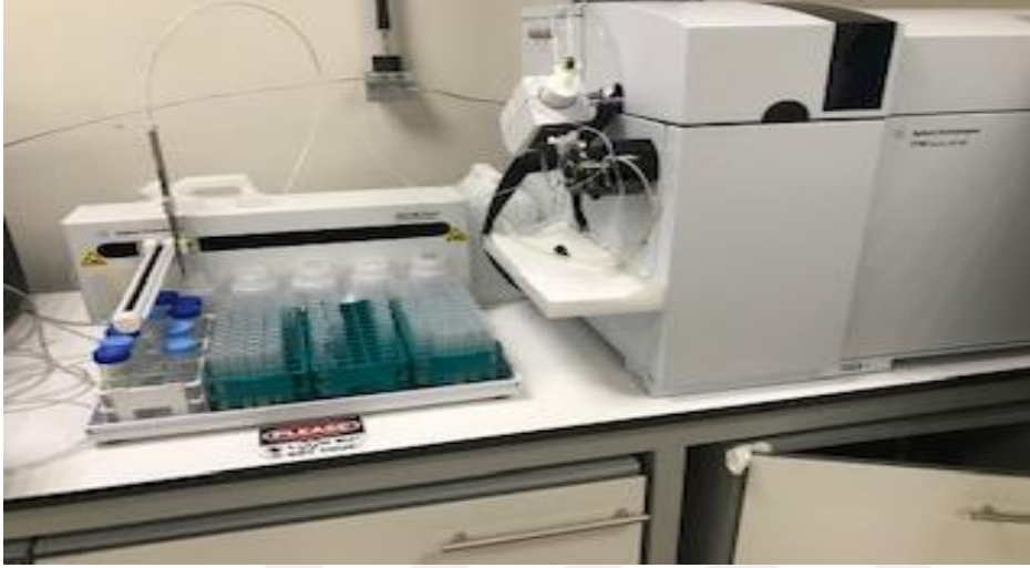
Şekil 3-8: ICP-MS cihazı (Agilent Technologies, 7700 series ICP-MS, ABD)
