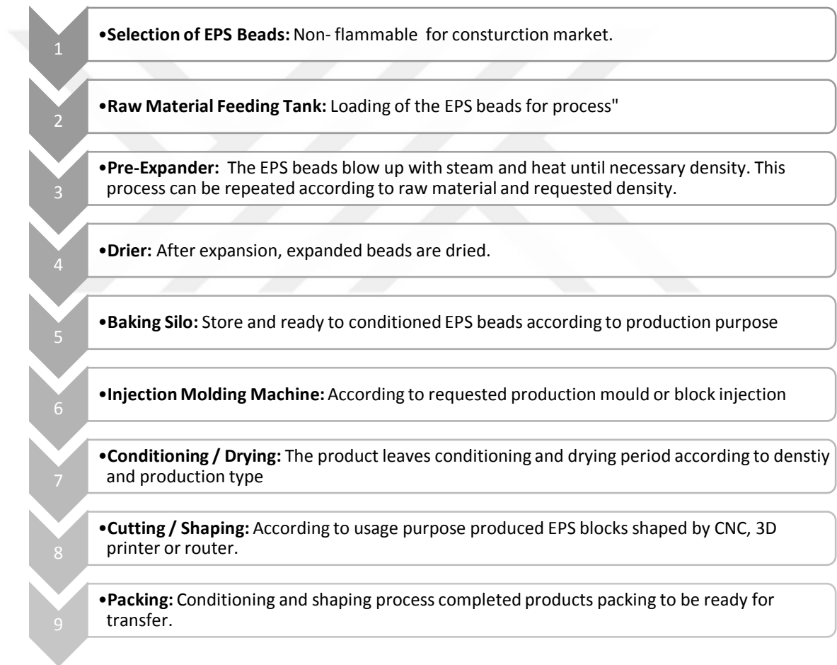
Figure 2. Production process of the EPS (by Erdemli)
