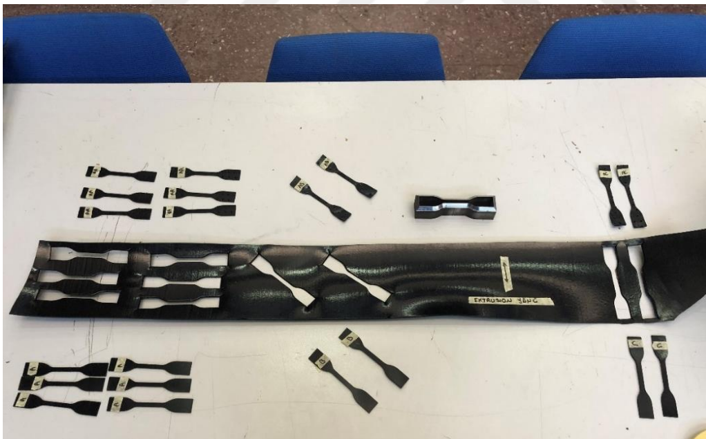
Figure 3.11 – Cut out HDPE ASTM D6693 tensile test specimens using a hydraulic press cut-out mold.
