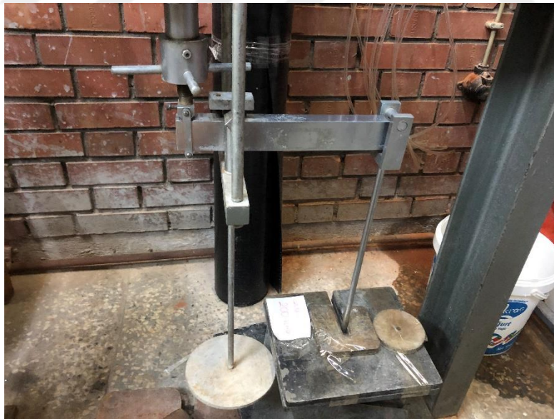
Figure 3.25 - Placement of leverage mechanism and pre-determined weight sets to the shearing device.
