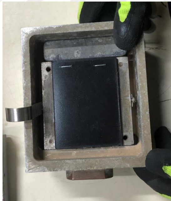
Figure 3.21 - A prepared, smooth HDPE geomembrane specimen placed in the direct shear box.
