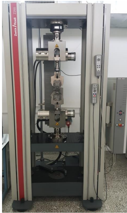
Figure 3.12 - Zwick/Roell Z250 Tensile Test Device
