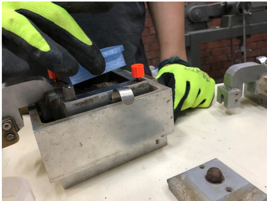
Figure 3.23 - Compression of the soil to the desired volume using a fixed height compression device.
