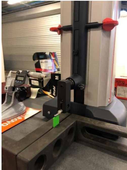
Figure 3.10 - Length measurement of tensile test specimens using linear height gauge and datum planes
