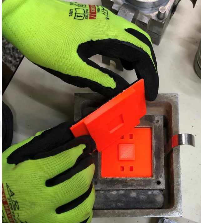
Figure 3.16 - Additively manufactured two-part assembly mounted on the direct shear setup.
