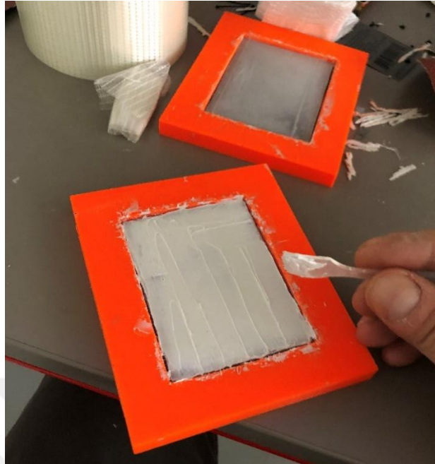
Figure 3.20 - The application of SMP glue to the geomembrane in the molds.
