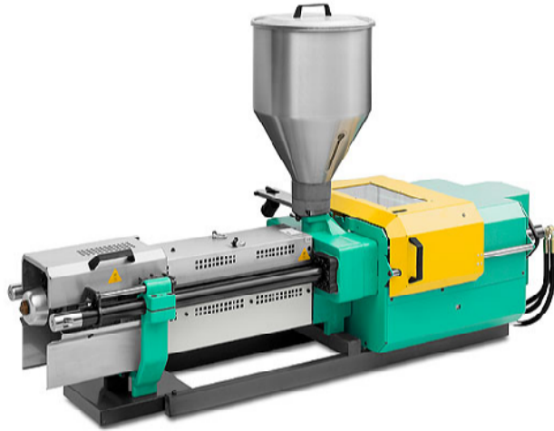
Şekil 3.21 Yatay enjeksiyon ünitesi ( http://www.arburg.com/com/COM/en/products/machines/standard/allrounder_u/injection_unit.jsp ).
