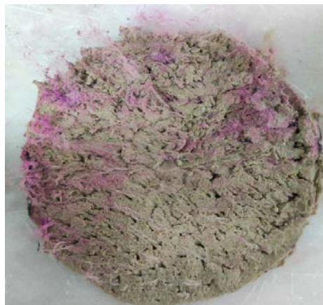
Figure 3.5 General view of M_b 3 after permeating with 15 mM \text{CaCl}_2 solution and dyed regions showing preferential flow paths after dye tests
