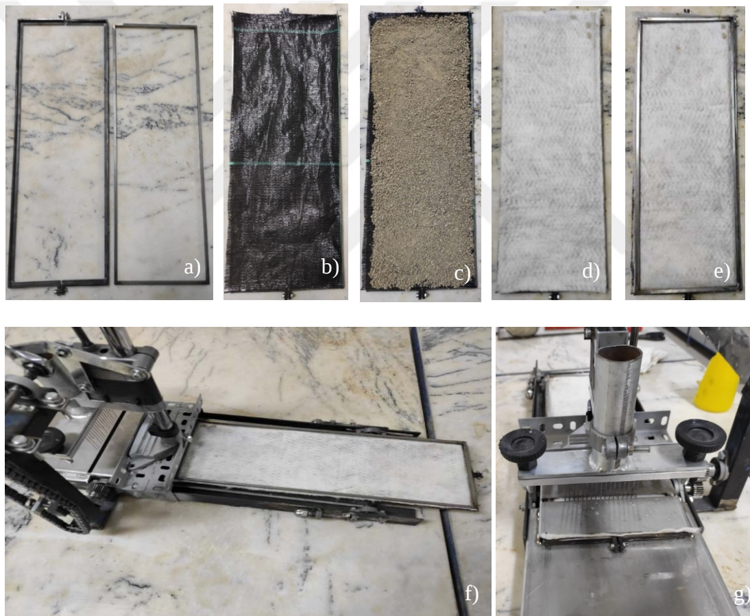
Figure 4.3 Photographs of A-GCLs during manufacturing: a) rectangular production frame, b) woven geotextile placed in the outer frame, c) bentonite placement on woven geotextile, d) non-woven geotextile overlying bentonite, e) placement of inner frame, f) sample ready for the needling, and g) manufacturing of A-GCL
