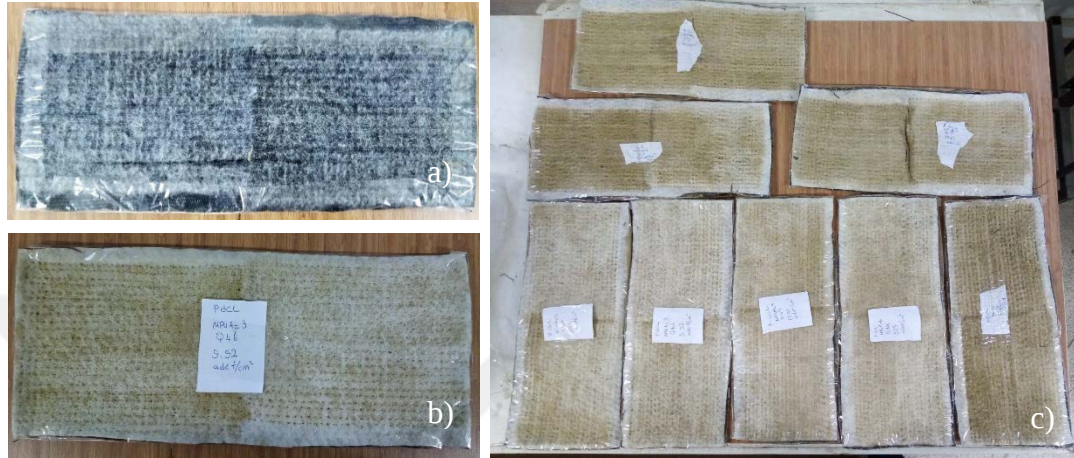
Figure 4.4 Appearance of A-GCLs after production: a) woven face, b) non-woven face, and c) other A-GCLs
