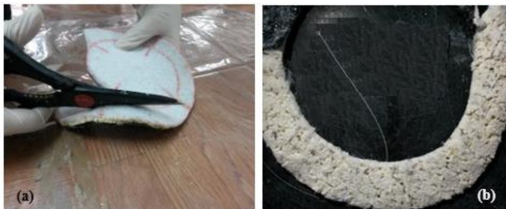
Figure 2.13 Sampling and monitoring of bentonite in SLSM after GCL: a) Cutting of GCL for hydraulic conductivity test, b) photographic image of swollen bentonite layer (Personal archive, 2015)
