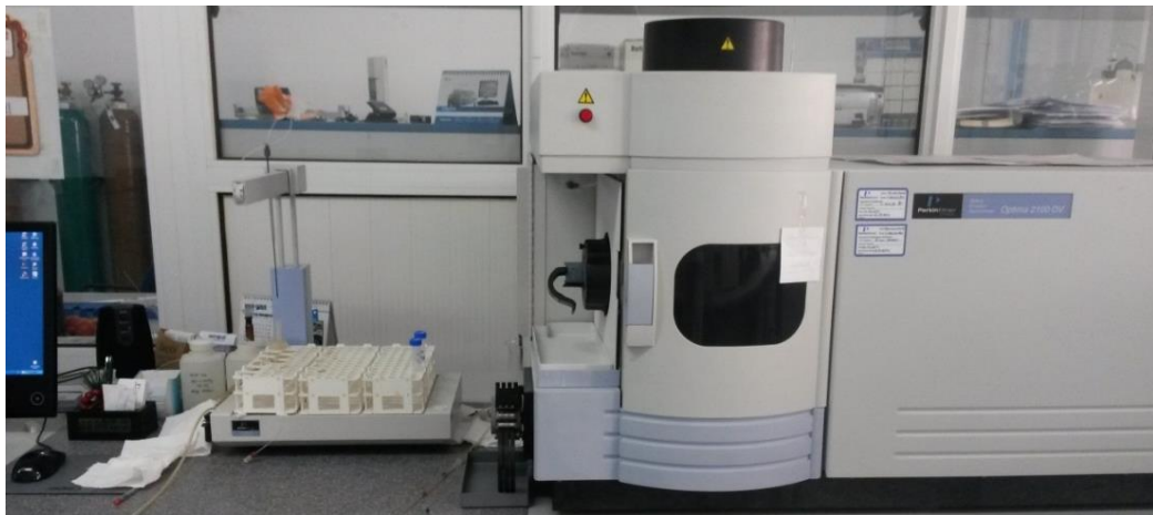
Figure 2.25 Pelkin Elmer DV 2100 Optima ICP-OES device that was used for the determination of cation concentrations in bentonites (Personal archive, 2017)
