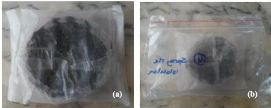
Figure 2.17 Storage of moistened or wetted GCLs: a) Wrapping with parafilm and b) kept into zipped bags (Personal archive, 2018)
