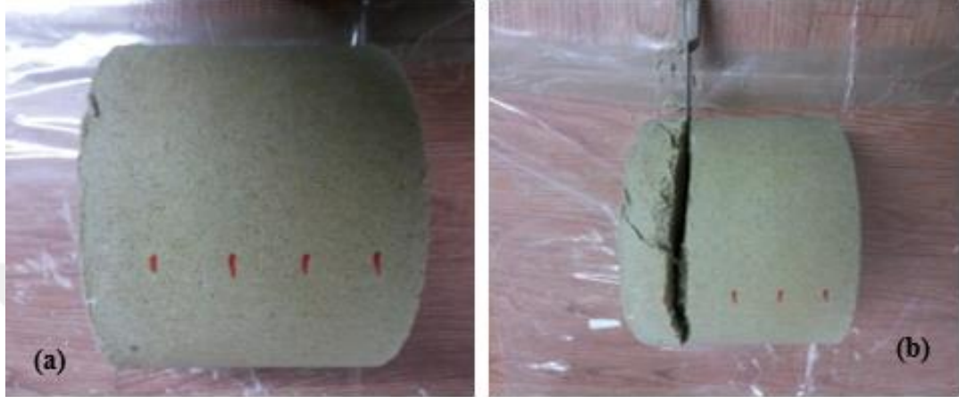
Figure 2.14 Subsoil after hydration: a) Marking the thicknesses; b) cutting the layers with spatula (Personal archive, 2015)
