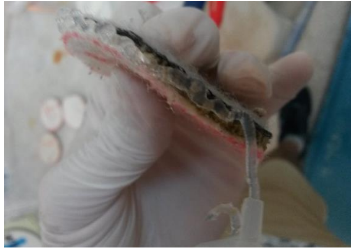
Figure 2.15 Photographic image of GCL sample during covering with silicone grease (Personal archive, 2018)
