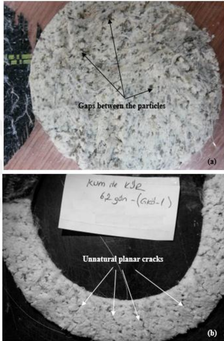
Figure 3.2 The picture of GCL-1 after 62 days of hydration with: a) CSM and b) SLSM (Personal archive, 2017)
