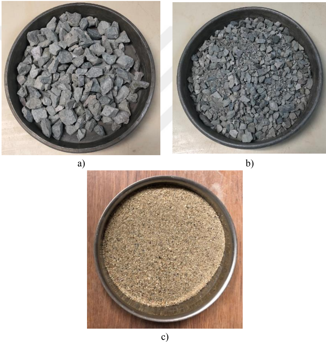
Figure 3.2 The photos of granular filter mixture materials a) coarse filter, b) fine filter and c) Çine sand
