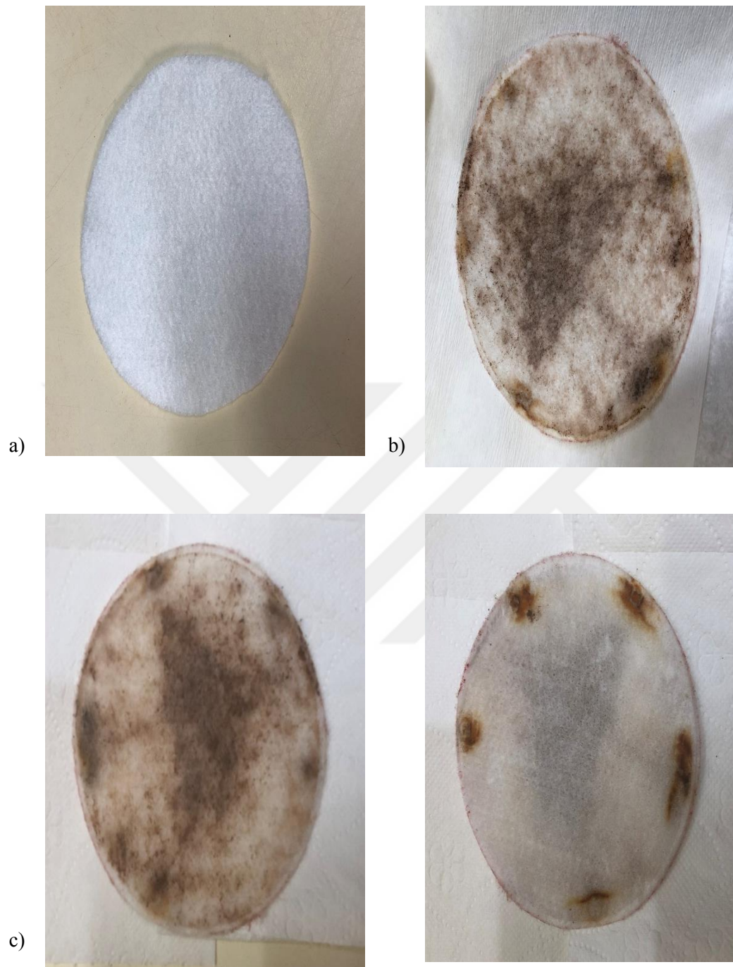
Figure 3.22 The photos of geotextile a) before the experiment T4, b) after the experiment T4, and c) after the experiment T5
