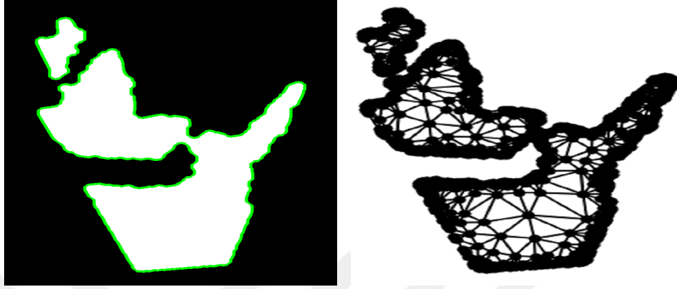
Figure 6.8: Example triangulation of the navigable area. The model image is preprocessed with erosion and dilation in order to refine it.
