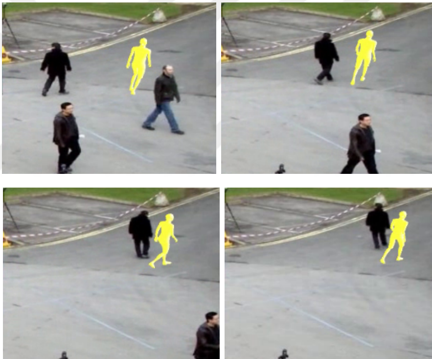
Figure 8.2: Sample interaction between an artificial agent and a detection in video. As the projected agents are unresponsive, the artificial agents are expected to take full responsibility for collision avoidance. In normal cases, both agents mutually change their velocities.
