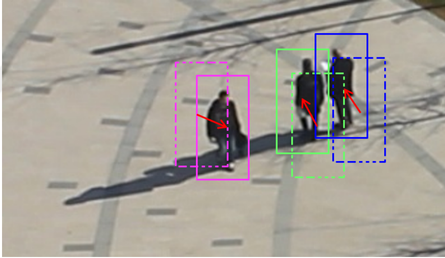
Figure 4.4: Using Kalman filters between consecutive frames, we are able to predict the next location of the tracked pedestrian and correct it according to detection in the next frame.
