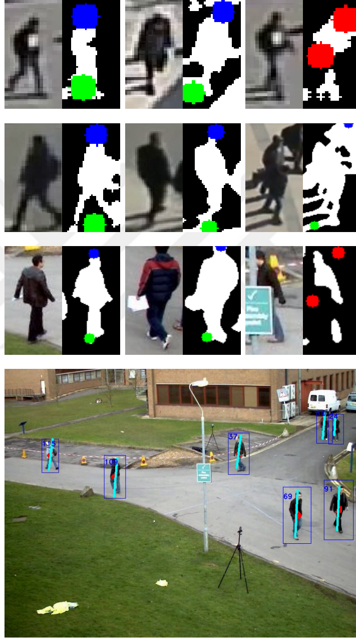
Figure 4.6: Example postures from different videos. Top three rows contain detections and corresponding foreground masks. Blue and green dots represent the rough position of the head and feet respectively. When legs are open: green points is the bottom point of the principal axis. Last column contains invalid postures, shown with red dots. In the middle row, rightmost posture is mistaken as a valid one, even though it contains multiple postures. At the bottom, each pedestrian together with their detection boxes (blue), unique tracking ID, posture line (cyan) and approximated direction arrow (red) is shown.
