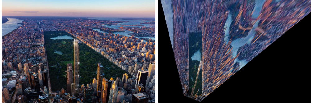
Figure 6.4: Example perspective correction of Central Park in New York, USA. This correction is performed using four point correspondences between image planes, which are the corners of Central Park. The image on the left is courtesy of ASGG and Wordsearch [78].
