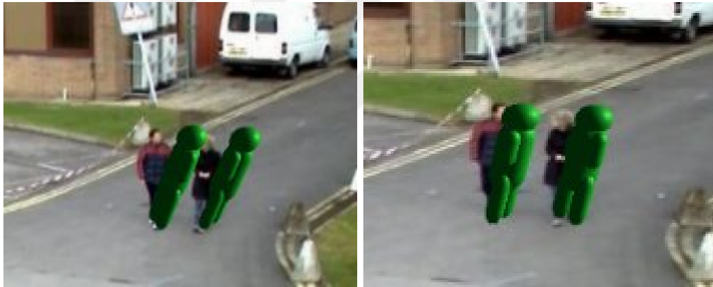
Figure 6.12: Differences in postures of dummy models with pedestrians in the video. A camera with a focal length smaller than expected will be placed closer to the area, resulting with the posture in the left figure. Better postures are obtained when the focal length approximation is more accurate.
