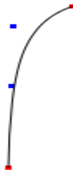
Figure 3.2: A strand produced by Bézier curve
