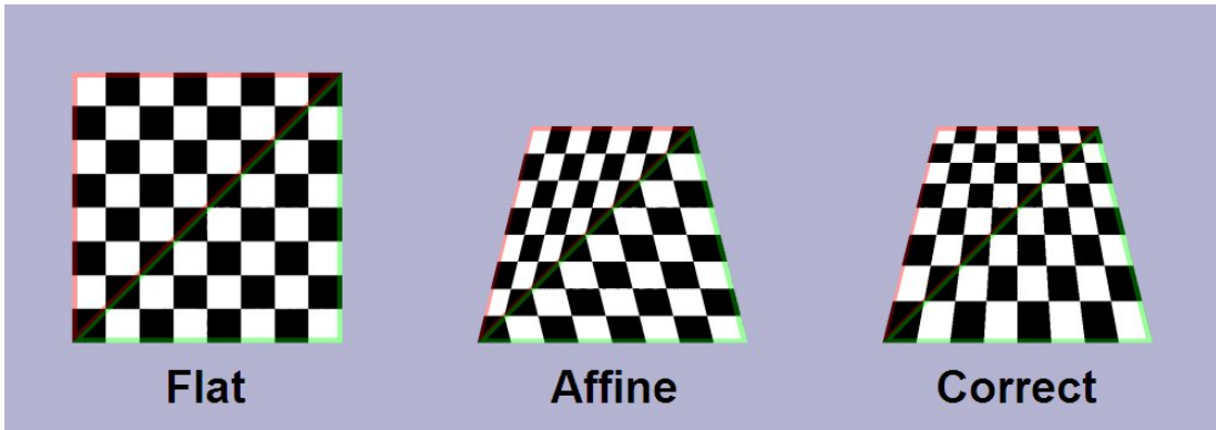
Figure 3.9: Difference between an affine (linear) texture mapping and a perspective corrected mapping. Wikipedia, “Texture mapping,” 2012. [Online; accessed 22-July-2012].
