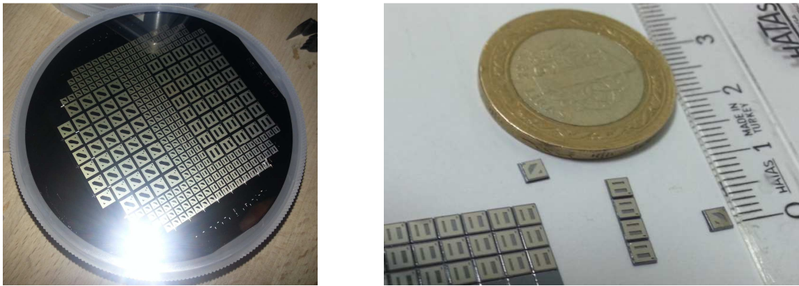
Figure 5.1: a) The wafer containing 2.5 mm x 2.5 mm chips b) the diced dies
