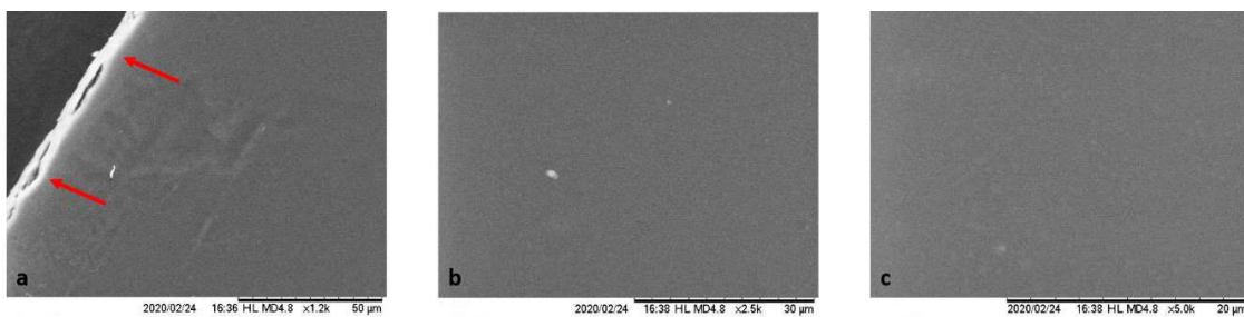
Figure 5.12. SEM images of D1 film at different magnifications a: 1.2 K X (The red arrows show the edge of the film), b: 2.5 K X, c: 5.0 K X
