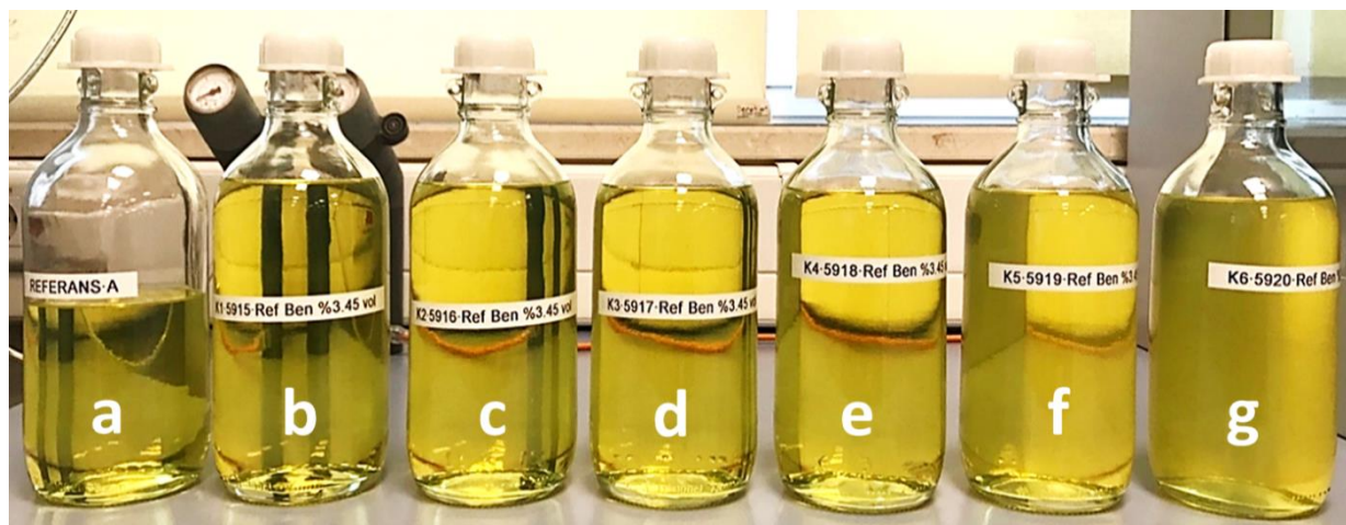
Figure 6-3. Appearance of a : the pure reference gasoline and b to g : its 3.45 vol% blends with the GTBE mixtures K1 to K6.
