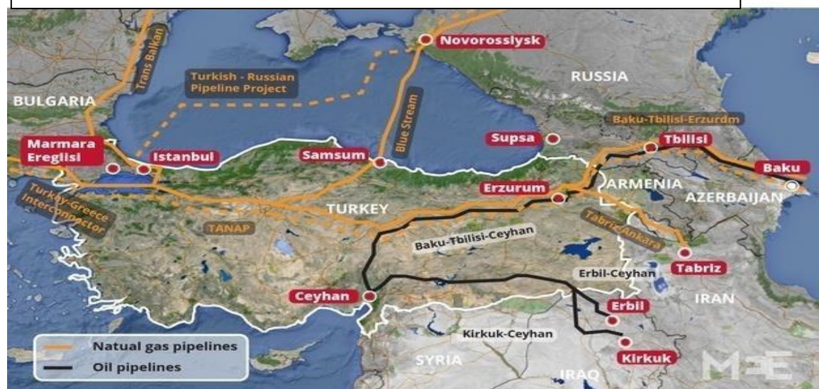
Figure 5.6.: Turkish Oil &amp; Gas Pipelines
