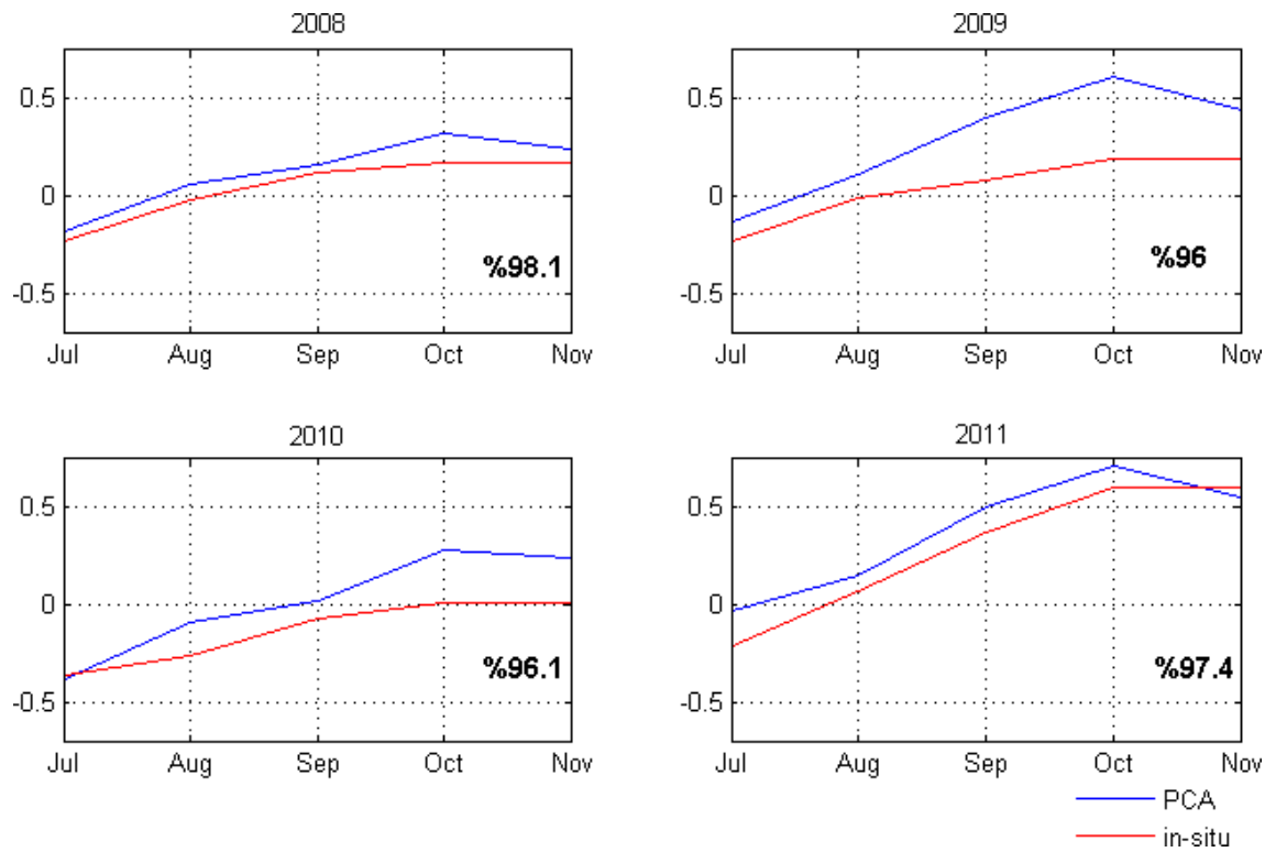
Figure 4.22: Most dominant mode of the time coefficients (principal components) is derived from CS3 GRACE solution (blue) and monthly average of in-situ data (red) of Mekong delta covering from 01.July to 30.November annual time period for year 2008 (left top), 2009 (right top), 2010 (left bottom) and 2011 (right bottom).
