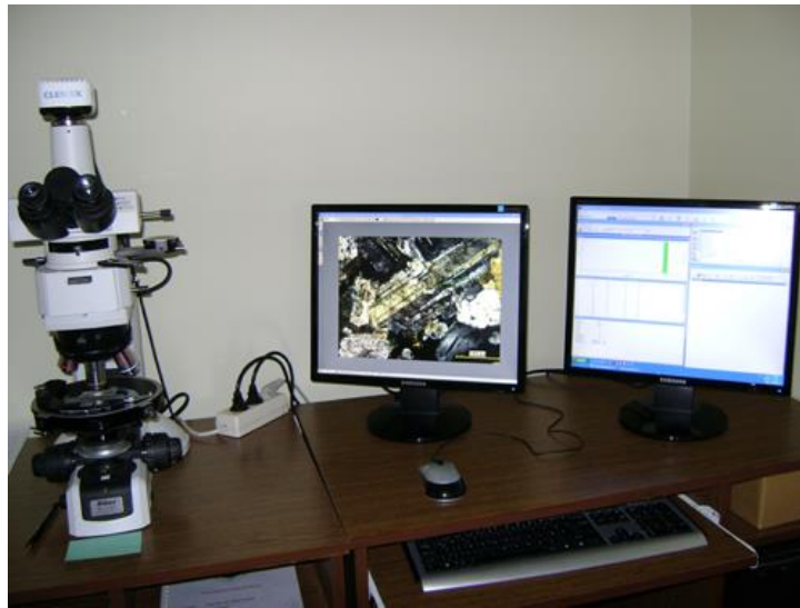
Resim 3.3 Nikon Marka Eclipse 2V100POL model mikroskop.
