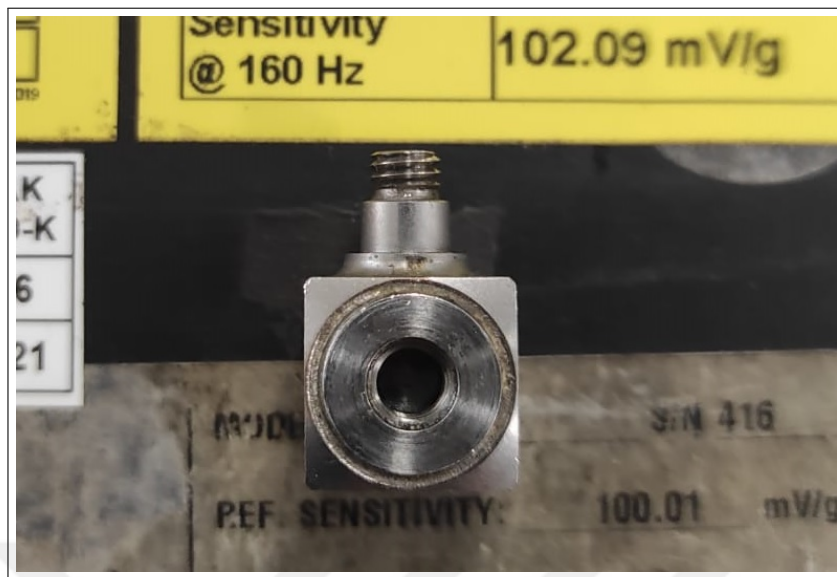
Figure 7.6. The accelerometer used for the mechanical experiment.
