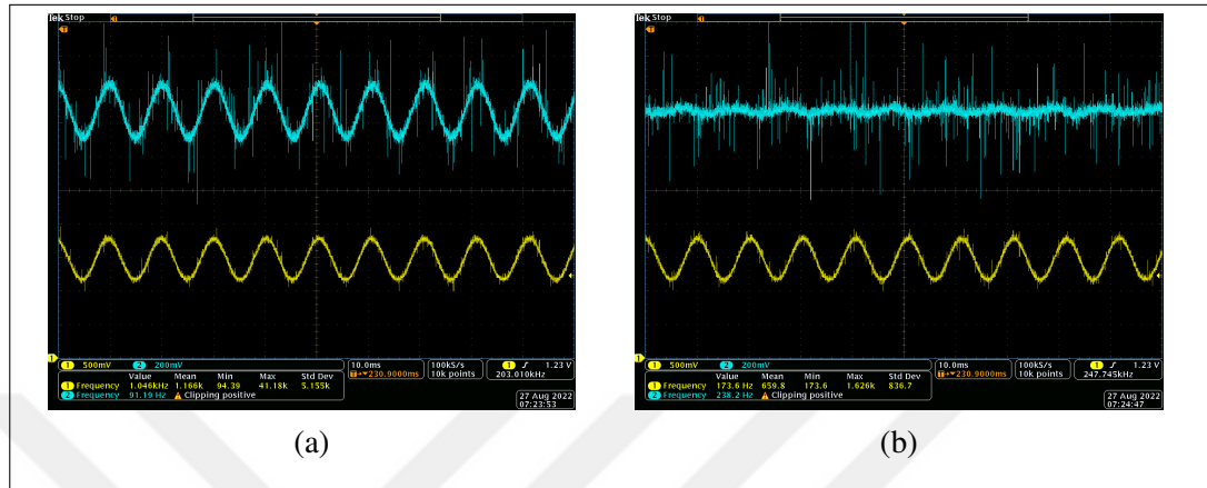
Figure 7.17. Obtained error and vibration signals when the PLL-based method (a) is not activated, and (b) is activated.
