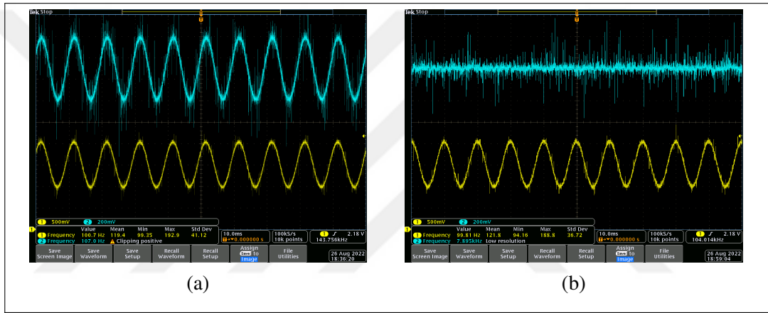
Figure 7.14. Obtained error and vibration signals when the proposed method (a) is not activated, and (b) is activated.
