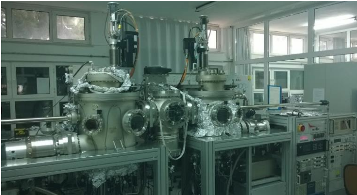
Figure 1.2. UHV Sputtering System (Anadolu University Advanced Technology Thin Film Laboratory)
