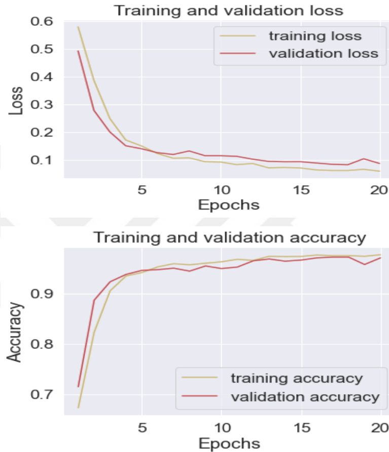
Figure 4.17. Training and validation accuracy and cross entropy loss of gray-scale hazelnut images with 20 Epochs
