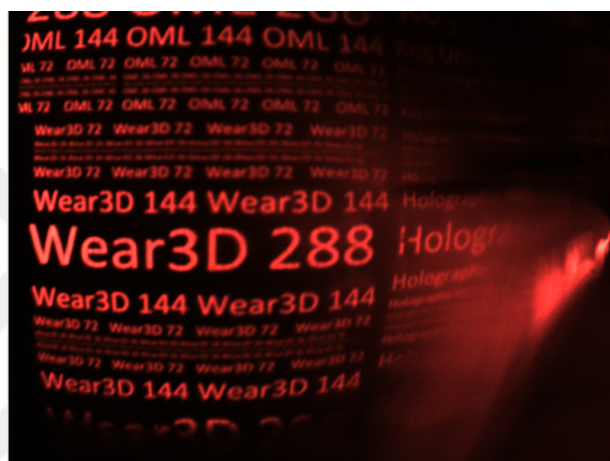
Figure 54: Image captured with ellipsoidal mirror while fiber is fixed with a syringe needle.
