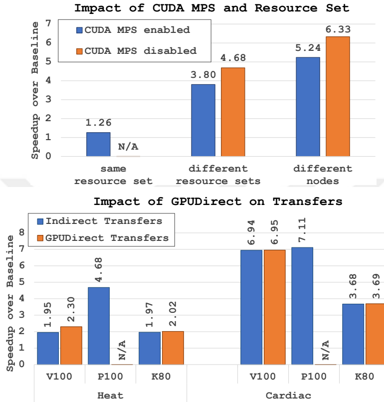
Figure 6.2: Performance impact of MPS, resource sets and GPUDirect on 4 GPUs
