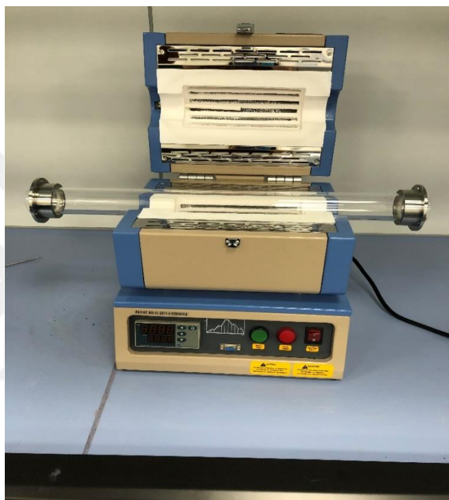
Figure 3.6: OTF-1200X-S50-2F mini CVD instrument.
