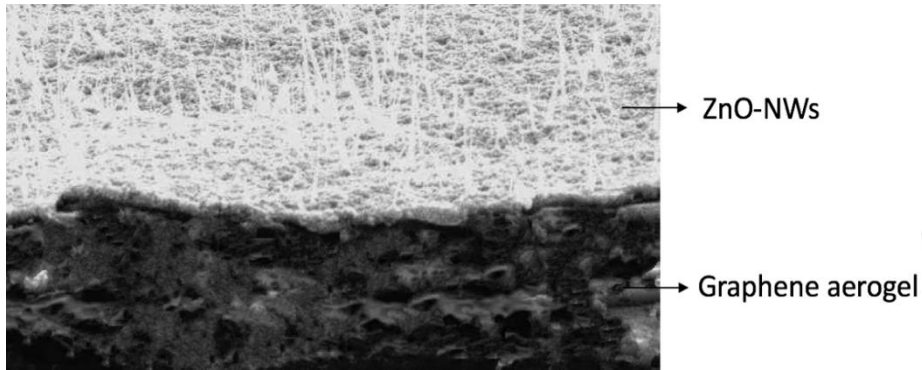
Figure 4.7: The cross-sectional FESEM image of the ZnO-NWs embedded in GA.
