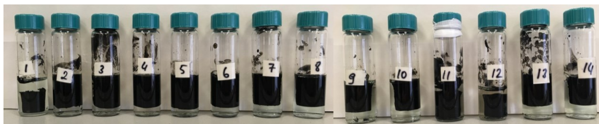
Figure 5-2 digital images of Ni/GA composites synthesized with various crosslinkers (1) 75 mM thiourea (2) 75 mM urea (3) 25 mM urea (4) 150 mM urea (5) 75 mM acetamide (6) 25 mM acetamide (7) 150 mM acetamide (8) glycine (Ni:gly=1:3 (mol)) (9) threonine (Ni:thr=1:3 (mol)) (10) alanine (Ni:ala=1:3 (mol)) (11) cystine (Ni:cys=1:1 (mol)) (12) L-cystine (Ni:cys=1:1.5 (mol)) (13) alanine (Ni:ala=1:2 (mol)) (14) threonine (Ni:thr=1:2 (mol)) after reaction at 95 °C for 24 h
