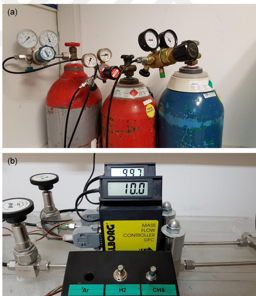
Figure 3.11 (a) The gases used during the growth are methane ( \text{CH}_4 ) as carbon source and hydrogen ( \text{H}_2 ) to anneal the copper surfaces.
