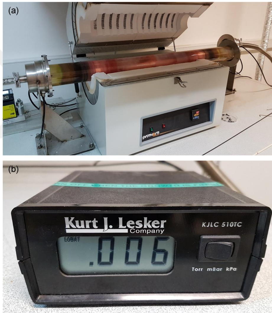
Figure 3.10 CVD system. (a) Furnace with quartz chamber, which can go up to 1070 degrees. The pump is used to vacuum the chamber. (b) Before the growth the chamber is vacuumed down to 3-6 mTorr.
