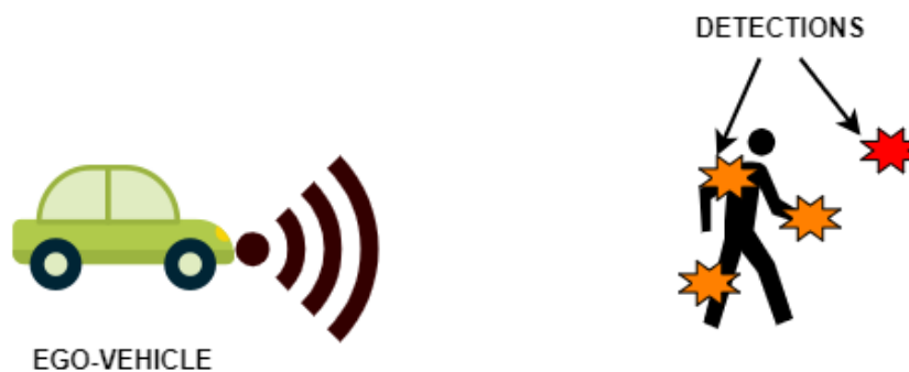
Figure 2.1 Depicting a host vehicle equipped with a RADAR system positioned at its front.
