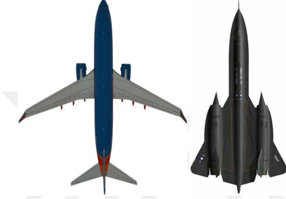
Figure 1.1. The difference in the configurations between a classic backward airplane (Boeing 737) and a delta wing aircraft (Lockheed SR71 Blackbird)
