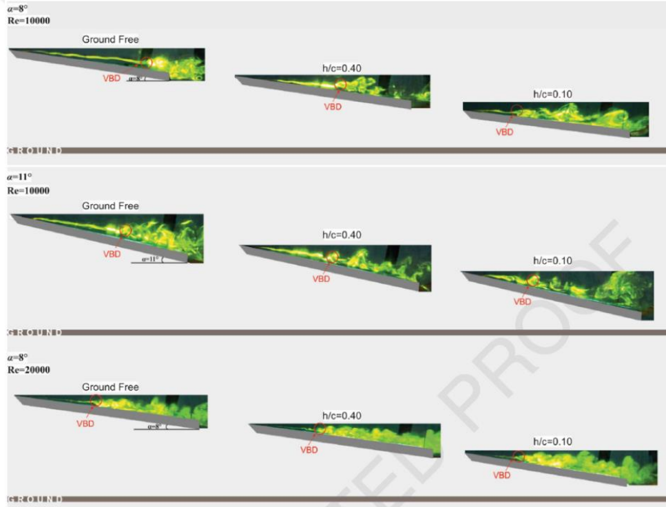
Figure 2.7. The ground effect on the location of vortex breakdown at \alpha=8^\circ and 11^\circ for h/c=0.1, 0.4 , and ground-free case (Tumse et al., 2021)
